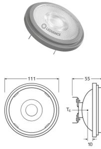
Specifications Ledvance SUPERIOR LED Spot Reflector G53 AR111 7.4W 450lm 24D - 927 Extra Warm White | Best Colour Rendering - Dimmable - Replaces 50W
