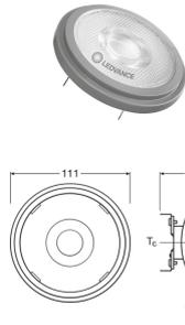
Specifications Ledvance SUPERIOR LED Spot Reflector G53 AR111 7.2W 450lm 40D - 918-927 Dim To Warm | Best Colour Rendering - Dimmable - Replaces 50W
